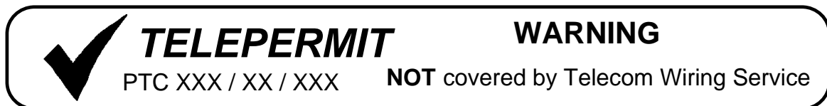
FIG. 4C TELEPERMIT LABEL FOR SPECIAL DESIGNS NOT COVERED BY TELECOM WIRING MAINTENANCE SERVICE
