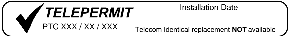
FIG. 4B TELEPERMIT LABEL FOR SPECIAL DESIGNS COVERED BY TELECOM WIRING MAINTENANCE, BUT NOT DIRECTLY REPLACEABLE
