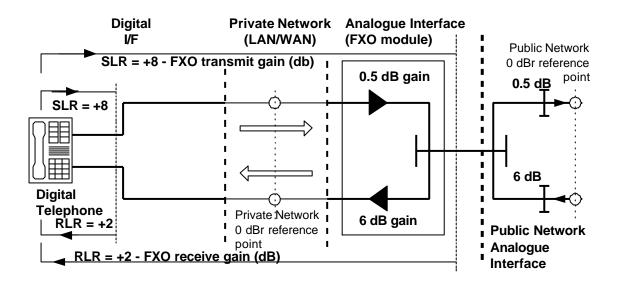
Send and Receive Loudness Ratings to be measured between IP Phone handset and 2-wire analogue network interface **Send Loudness Rating (SLR)** +11 dB to +2 dB, **Objective: +5 dB**
