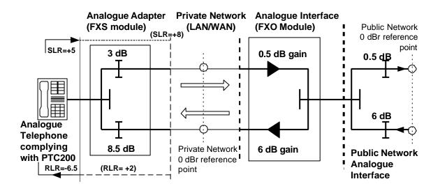
Loss from FXS port to FXO port: 1 to 5 dB, **Objective: 2.5 dB** Loss from FXO port to FXS port: 1 to 5 dB, **Objective 2.5 dB**
