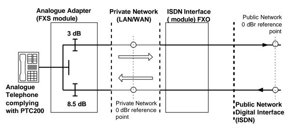
Loss from extension port to ISDN: 1 to 5 dB, **Objective: 3 dB** Loss from ISDN to extension port: 6.5 to 10.5 dB, **Objective 8.5 dB**
